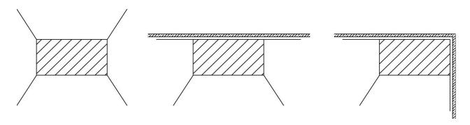
If the staircase is placed against a wall, do not remove the expansion leg/arch, but turn it parallel to the wall. If the staircase is placed in a corner, remove the inner expansion leg/arch, and turn the outer two parallel to the wall.
