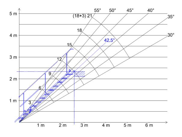
Example 12 treden trap Height: 2.350 mm Distance: 2.550 mm Degrees: 42,50
