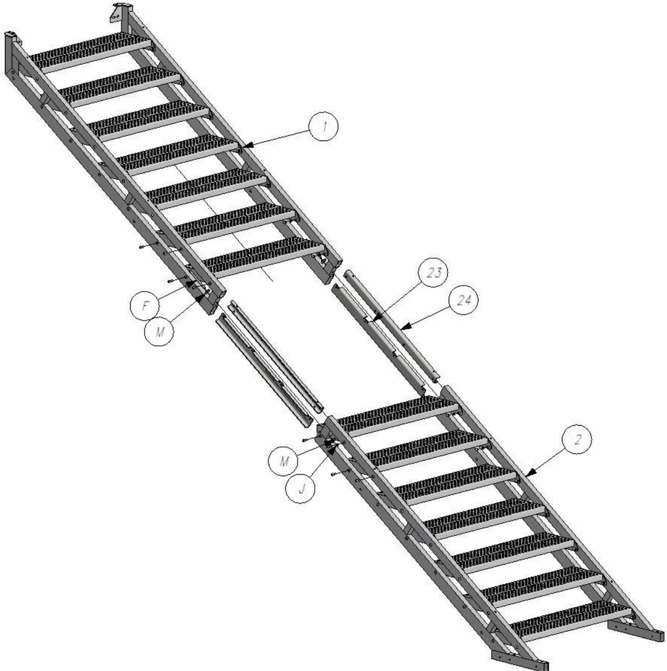
The posts, which are installed next to the stairs should be screwed to the inner side of the platform with the same screws as the stairs.
