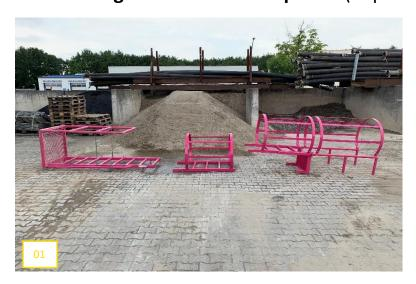
01 The standard version of the cage ladder is 4.00 m long. (Load capacity 185 kg)
