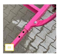
03 The intermediate pieces are connected with 4 M12 screws each (SW19, thread min. 8.8) with self locking nuts.
