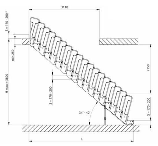
The above example is using ASTA-UL4 and ASTA-UL5 brackets.
