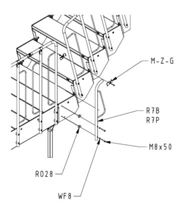
Railing with FI 12 mm tubes (C) & railing with FI 4 mm lines (C\*)
