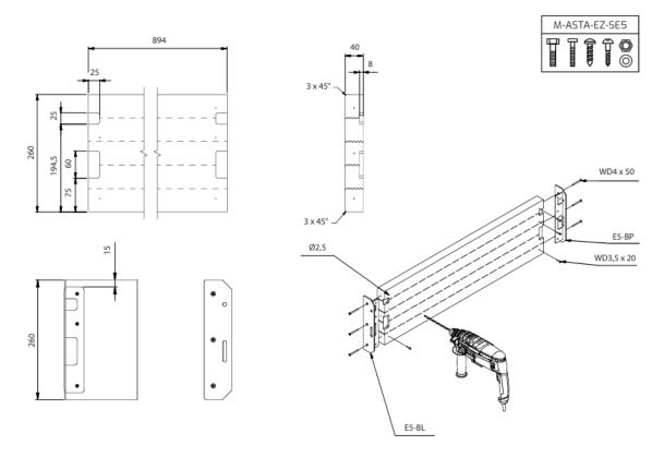
Wooden steps assembled on steel substructure (variant E2, E3, ER).
