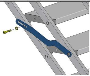
In order to ensure the rigidity of the staircase, the bolts securing all locks must be tightened. Tighten connections with approximately 60% of the tightening torque prescribed for the diameter and class of connector.
