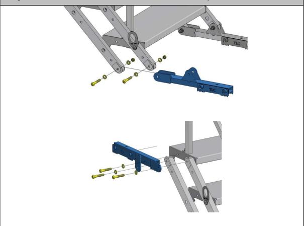
Removing the L30 handle connector, unscrew the bolt fixing the handle, pull off the handle, pull out the sleeve, screw in the bolt. Note: bot screwing in required.
