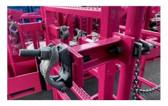
The clamps that are in the middle of the lower part of the sheet pile ladder are folded out. Attach these to the intermediate pieces.
