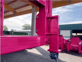
Before lowering the ladder, the support posts and clamps should be slid into the desired position. Note: Distance to the wall should be at least 150 mm for sufficient stability.
