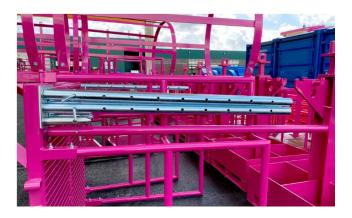
The lower platform contains the mounted holders for the tubes.
