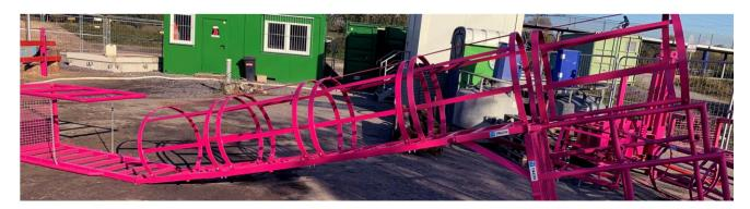
The length of the sheet pile ladder can be adjusted by means of a screw system. The 1.000 mm long intermediate pieces (40 kg) extend the sheet pile ladders to a maximum of 10.000 mm.
