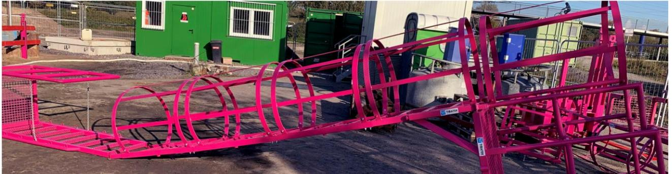
The length of the sheet pile ladder can be adjusted by means of a screw system. The 1.000 mm long intermediate pieces (40 kg) extend the sheet pile ladders to a maximum of 10.000 mm.
