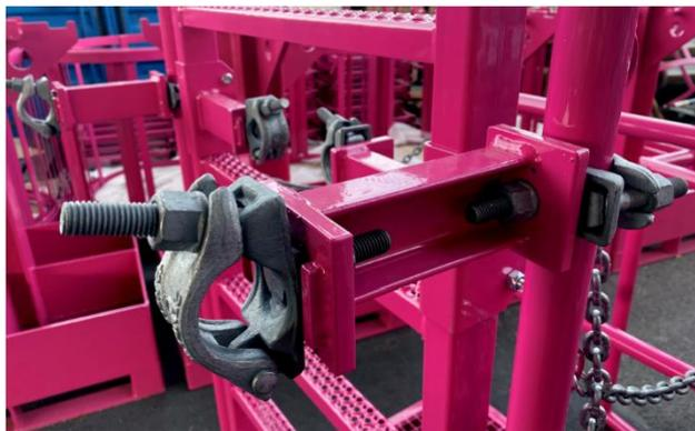
The clamps that are in the middle of the lower part of the sheet pile ladder are folded out. Attach these to the intermediate pieces.
